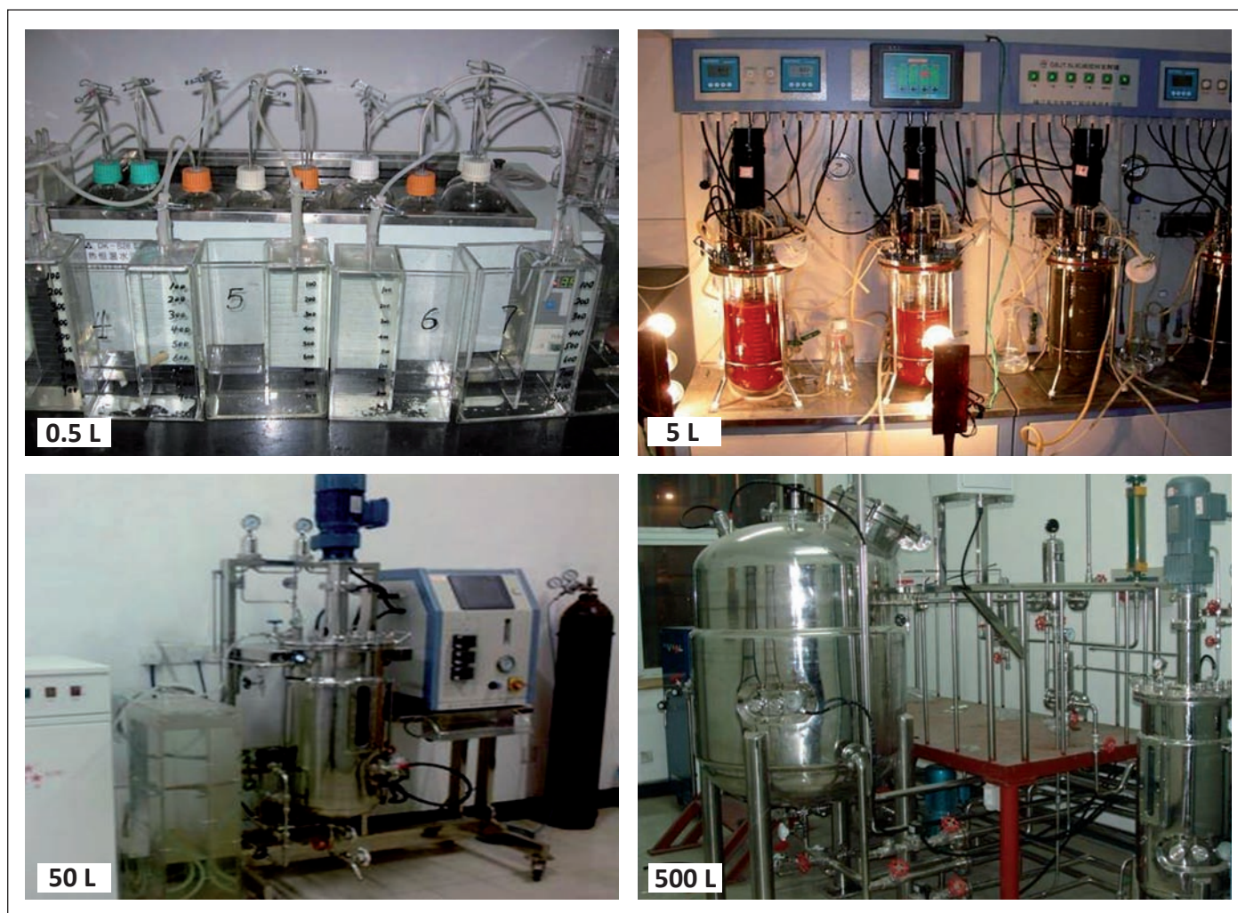
Apparati for fermentative H_2 production from microalgae. Photos: J. Cheng
