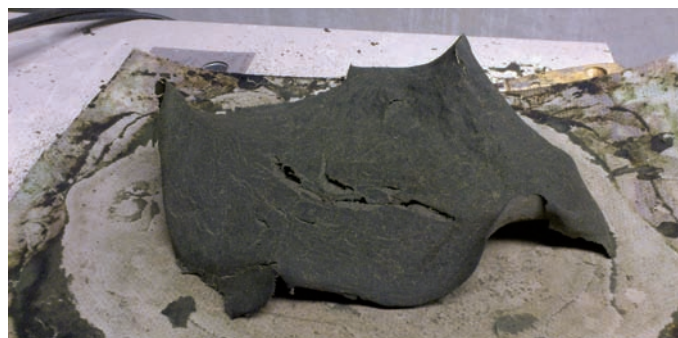
Dry algae biomass produced in the photobioreactor. The algae were grown on urban wastewater and flue gases. Photo: F. Gentili
