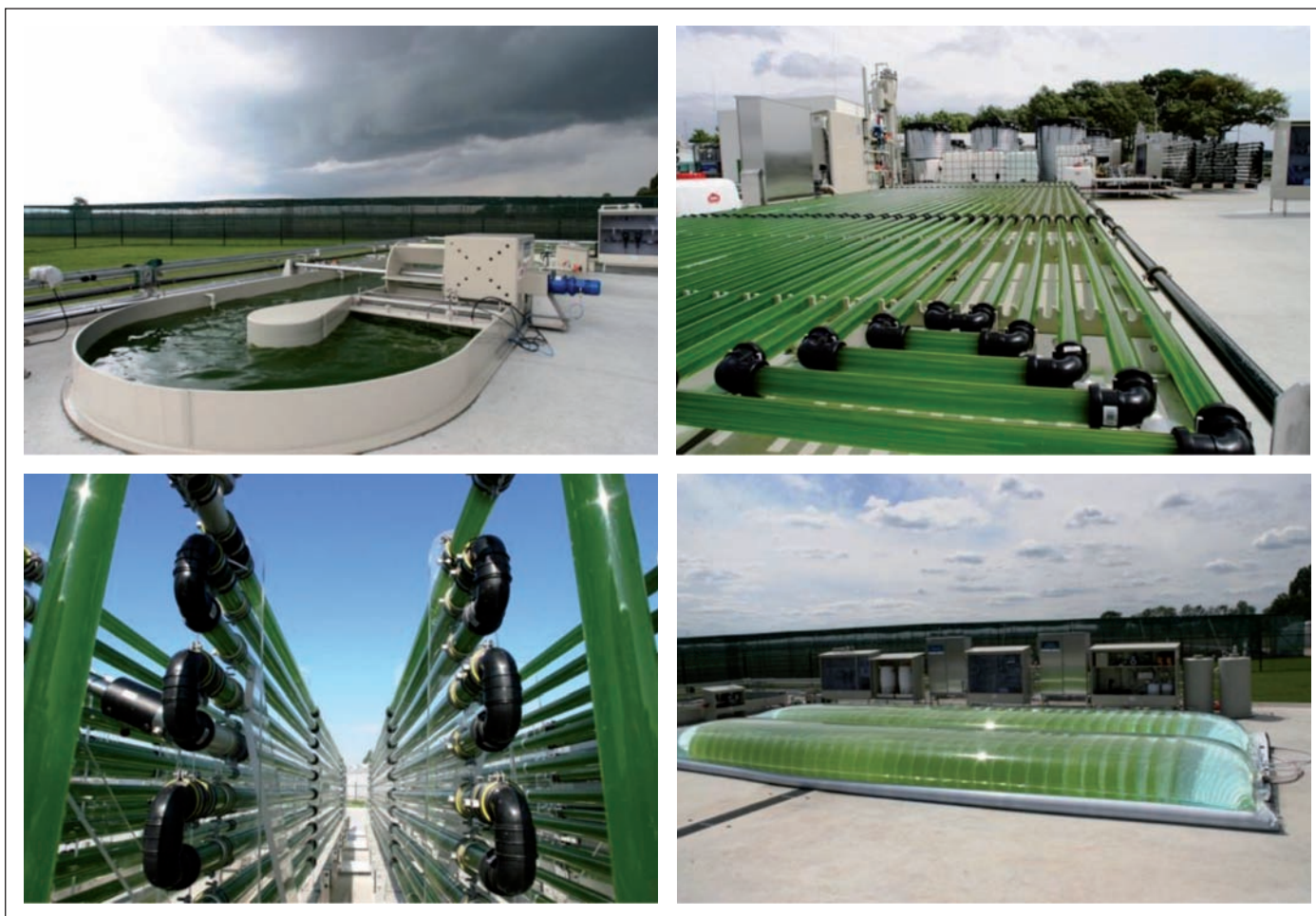
The four types of reactor systems at AlgaePARC (left to right, top to bottom): open raceway pond, horizontal tubular reactor, vertically stacked tubular reactor and flat panel reactor. Photos: AlgaePARC
